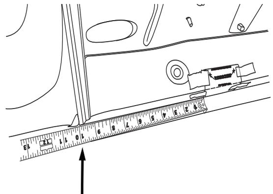
Pre Drill holes with an 1/8" Drill and then drill to 17/32". Then insert rivet nuts into position. Refer to install card in rivet nut tool bag. Then pre thread m8 screws and washers into position
