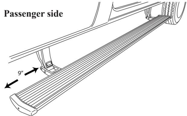
Install Running board onto lower mounts. Measure 9 inches from end of board to side of linkage as shown below.
