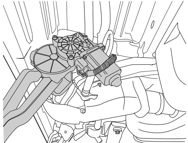
Run harness end up through the large rubber boot. Zip tie around boot may need to be removed to route wire through. If so use one supplied and re-seal boot.
