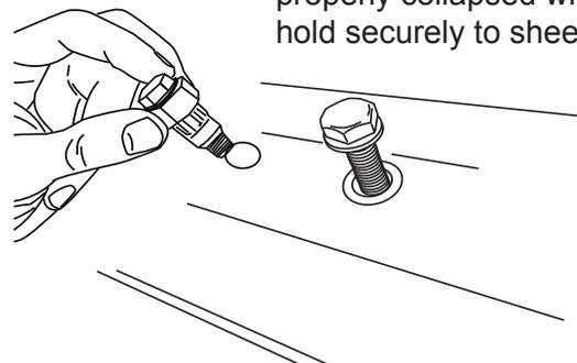
**Warning:** Rivet nuts not properly collapsed will not hold securely to sheet metal.
