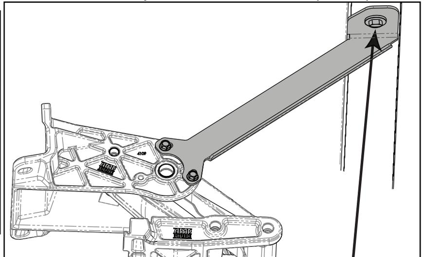
To attach the **Rear Bracket** (#21) to the rear linkage, start by using the Thread Cutting bolt (#23), to cut threads in the blank insert in the frame rail. Use a 9/16" socket and ratchet, go slow and stay straight. Then install the bracket on the non-motor side of linkage loosely with two bolts (#22), install the upper Bolt (#23) and Washer (#24), loosely and tighten the bottom two bolts fully. Now, tighten the top.
