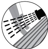
**Maintenance:** In adverse conditions, debris such as mud, dirt, and salt may become trapped in the running board mechanism, possibly leading to unwanted noise. If this occurs, manually set the running boards to the deployed position and flush the front and rear hinge arms with a high-pressure car wash wand.
