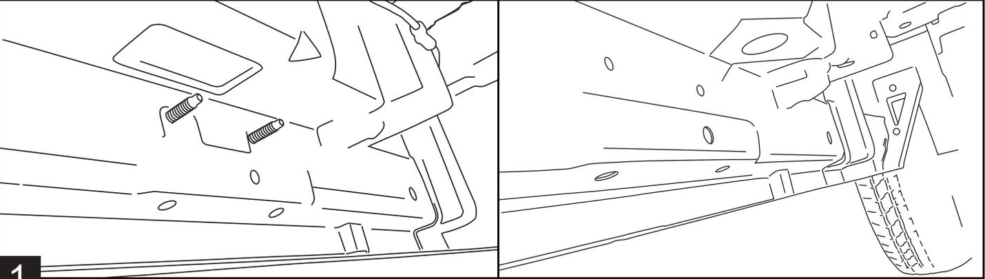
To attach the **Rear Motor Linkage** to the rear factory-step mount location, when no studs/threaded inserts are present, the three holes need to be drilled to the proper size **17/32"** to install three Rivet nuts (#7) using the supplied Rivet nut tool (#16). Next, install the **Rear Motor Linkage** (#3) using three Conical bolts (#6),
