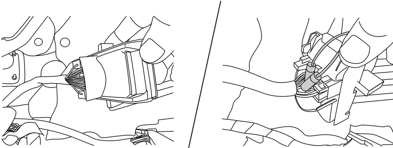
Once the trigger wire has been connected to the OBDII module (#18), remove the OBDII port from the vehicle by depressing the two plastic tabs on the sides and push the port back out of the bracket. Now connect the OBDII module to the OBDII port.
