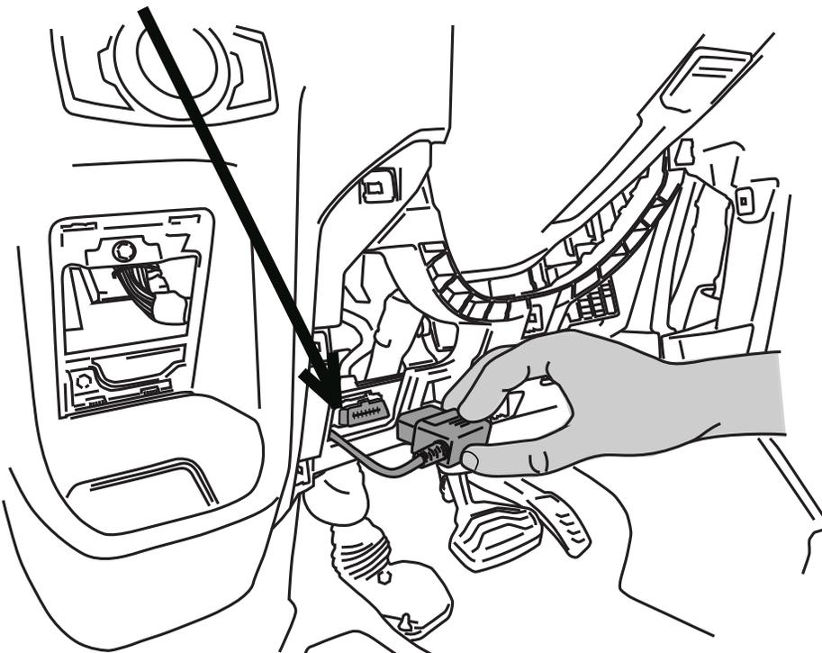
**OBD II install:** Use Supplied Posi-Lock™ connectors to attach the Plug and Play Module to the Harness. Attach matching colors on the harness to the wires on the module. Plug in module to OBD II port on the vehicle. Secure harness with supplied tie wraps. *Note: If the OBD II pass thru harness (76404-01A) was purchased see install sheet supplied in packaging. The pass through harness allows for an open port for other accessories. See below for a brief description.*
