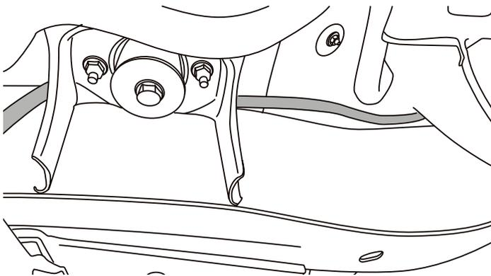
**On the Driver side, Do Not Ziptire the Wire Harness to the Brake Lines.**
