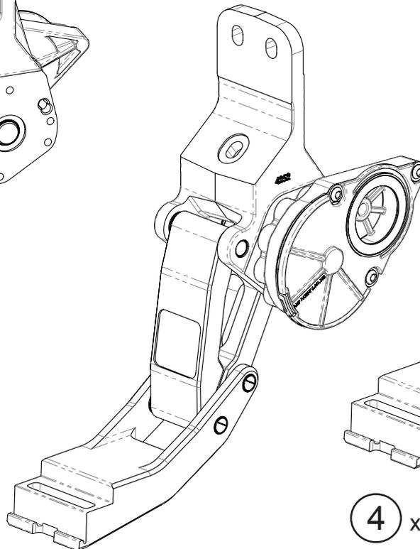
③ Passenger Motor Linkage Assembly
