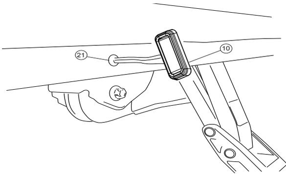
Insert grommet(21) into drilled holes. Insert lamp(10) wires through the grommets. (Silicon lube will help wires slip through grommets.)
