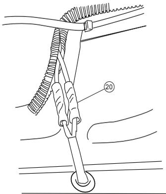
Using supplied butt connectors, connect the lamp wires. Red to Red, Black to Black. Once Crimped use heat gun to shrink tube.
