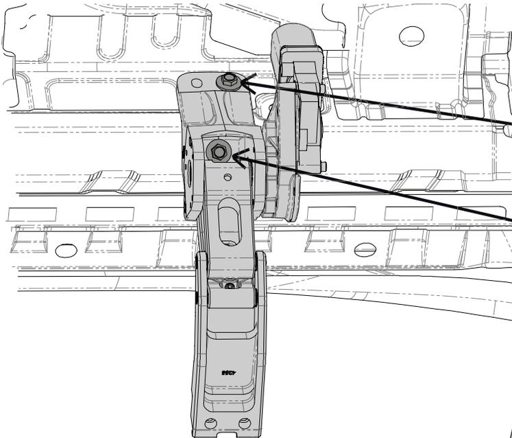
Assemble the motor to the linkage like the diagram below before installation. Position the motor so the linkage is in the most extended position.
