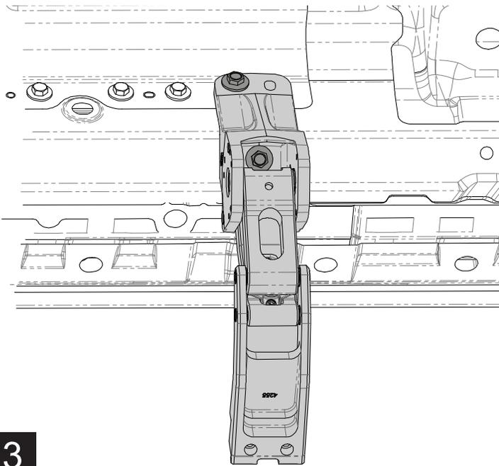
Next, install the Idler linkage in the **Third mount position from the front of the truck. Install the upper bolt in the rearward hole.** To install the lower bolt, put the bolt in a socket on an extension to guide it into position. Keep the linkage held up to the angled surface and vertical surfaces while tightening the bolts. **Torque fasteners to 16 ft-lbs. (22 N m).**
