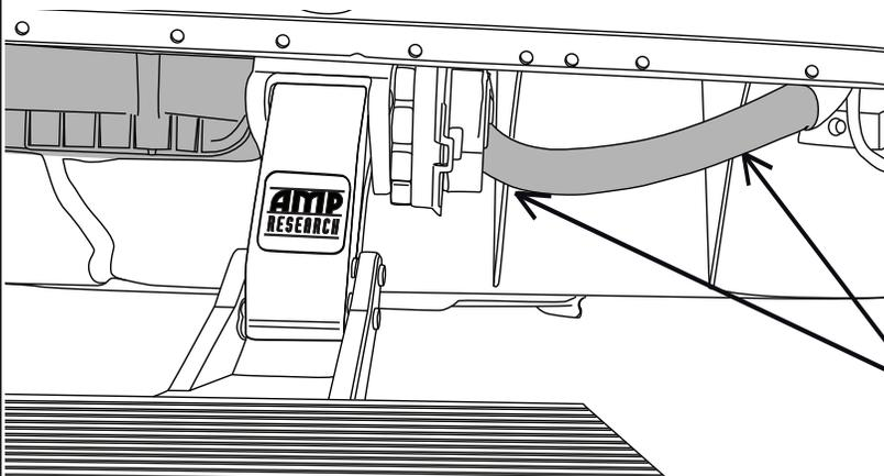
Assemble the motor to the linkage like the diagram below before installation. Position the motor so the linkage is in the most extended position.
