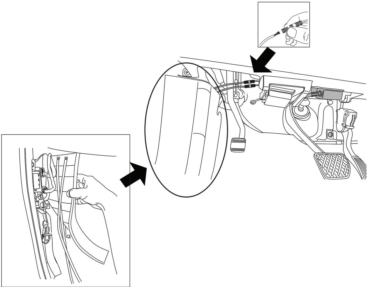
Use the Posi Locks(11) to make the connection to the plug and play module. Next plug in the Plug and Play(7) module under the dash as shown and route the wires behind the hood latch to the left. Make sure the wires are clear of the E-brake mechanism when it is on and off. The wires from below can be tucked under the carpet and covered with the trim reinstated. Then reinstall the trim.
