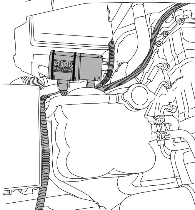
Next, connect the Black wire to the ground screw on the inner fender in diagram at top of page. Connect the Red wire to the stud on the positive power battery cable terminal.
