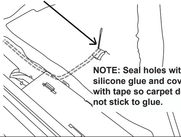
**NOTE: Seal holes with silicone glue and cover with tape so carpet does not stick to glue.**
