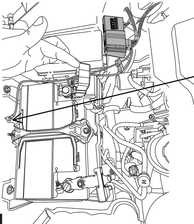
Next, connect the Black wire to the chassis ground screw on the inner fender behind the battery. Connect the Red wire to the stud on the positive power battery cable-terminal.
