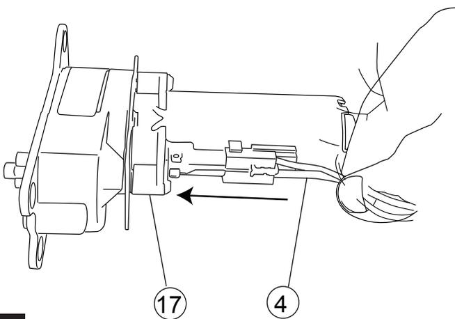
Slide rubber grommet on Wire Harness into slot of Motor Cover. Slide Motor Cover over Motor.
