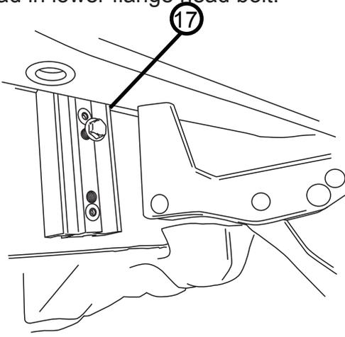
Snug bolts to allow for adjustment at a later step.
