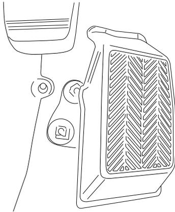
Pry up front door sill plates and remove kick panel fasteners and panels on driver and passenger side.
