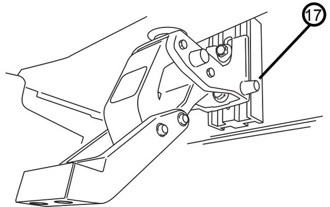
Locate Rear most set of threaded holes on the frame just forward of rear suspension. Vehicle shown has Vehicle Stability Control lines. Tighten screws to 16 ft-lbs.
