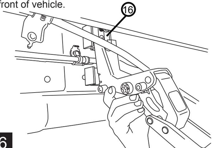
Slide mounting T-nut into position. Slide the board back so that the front of the board is aligned with the front edge of the front door. Torque to 10 ft-lbs.
