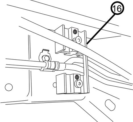
Pre thread upper M10 flange head bolt onto frame mount. Slide linkage into position and thread in lower flange head bolt. Motor faces front of vehicle.
