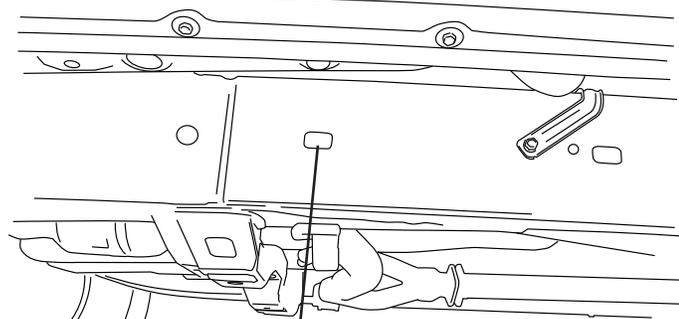
Through-bolt linkage to frame using this hole.
