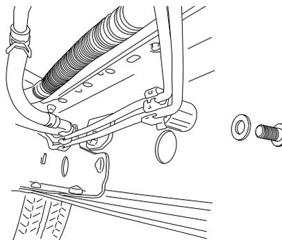
Replace all brake line fasteners.
