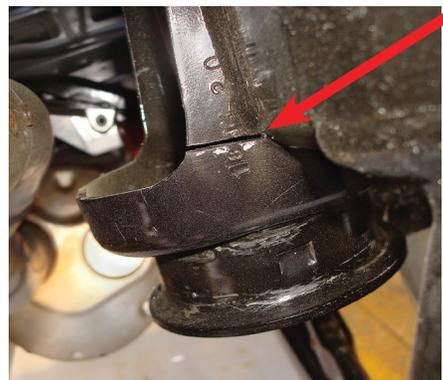
Cut the jounce bumper bracket to level above the bottom of the frame. Do not cut into the frame. Passenger's (right) side shown.
