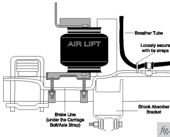
7. Using the holes in the upper bracket as a template, drill two 5/16" holes into the frame. Insert and tighten the self tapping bolts (K) and torque to 15 ft-lbs. (Figures 1 and 7).
