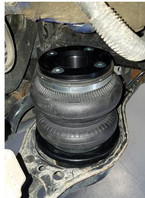
7. Center air spring assembly in lower control arm spring pocket (Fig. D.31). Install centering spacer (J) with M10-1.5 x 90 hex cap screw bolt (K) and M10 split lock washer (H) (Fig. D.32) and torque bolt to 46Nm (34 lb.-ft.). Ensure air line and fitting are still pointing inboard toward pivot point before torquing bolt.
