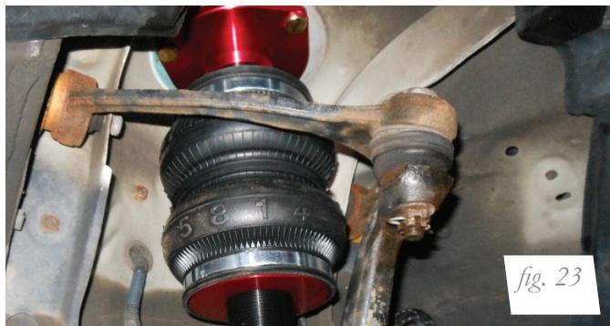
5. Reassemble the stabilizer bar to the stabilizer bar end link (fig. 24). Torque both the nut and bolt to 55Nm (43lb-ft).
