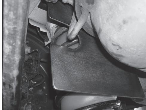
Make sure the slot in the heat shield is around the muffler mounting bracket.
