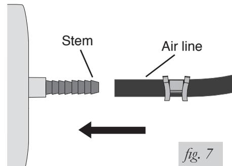
7. Slide the air line clamp over the air line. Push the air line onto the fitting covering all barbs. Using pliers, slide the air line clamp forward until it fully covers the barbed section (fig. 10).
