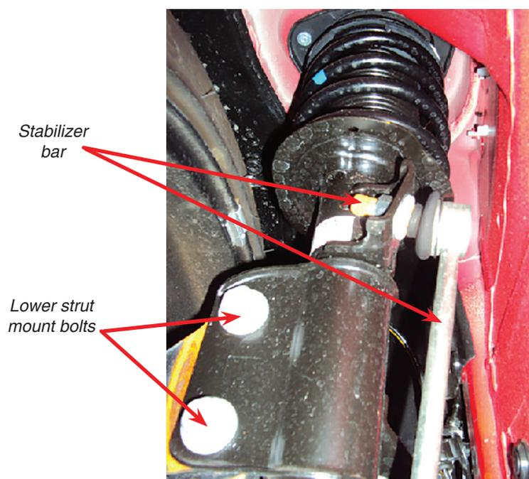
3. Support the hub then unbolt and remove the two lower strut mount bolts (fig. 3).
