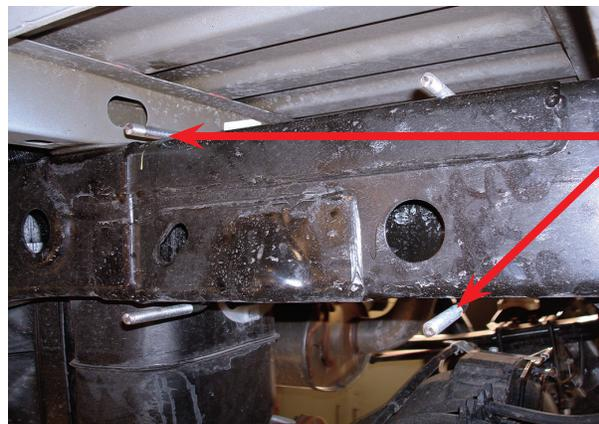
Figure 7 shows the left (driver-side) outside frame with the U-bolts in position.
