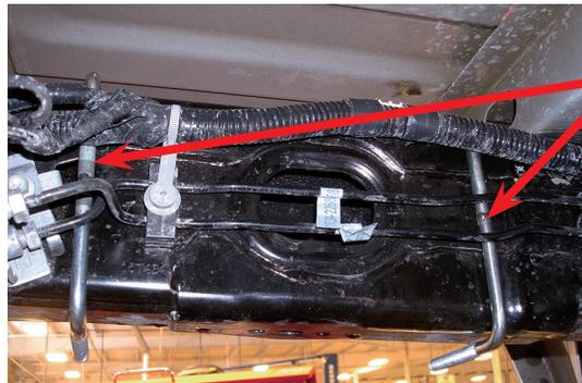
Figure 6 shows the U-bolts in the proper location, under the brake lines and wiring on the inside of the left side frame (driver-side).
