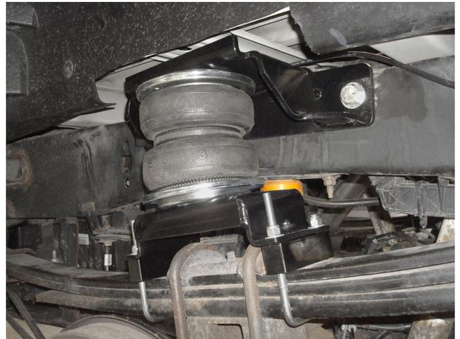
Rear axle view of driver's (left) side installation.
