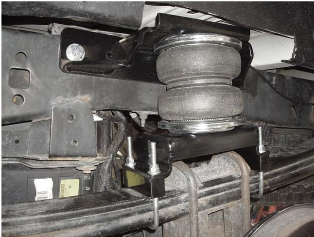
Forward of axle view of driver's (left) side installation.
