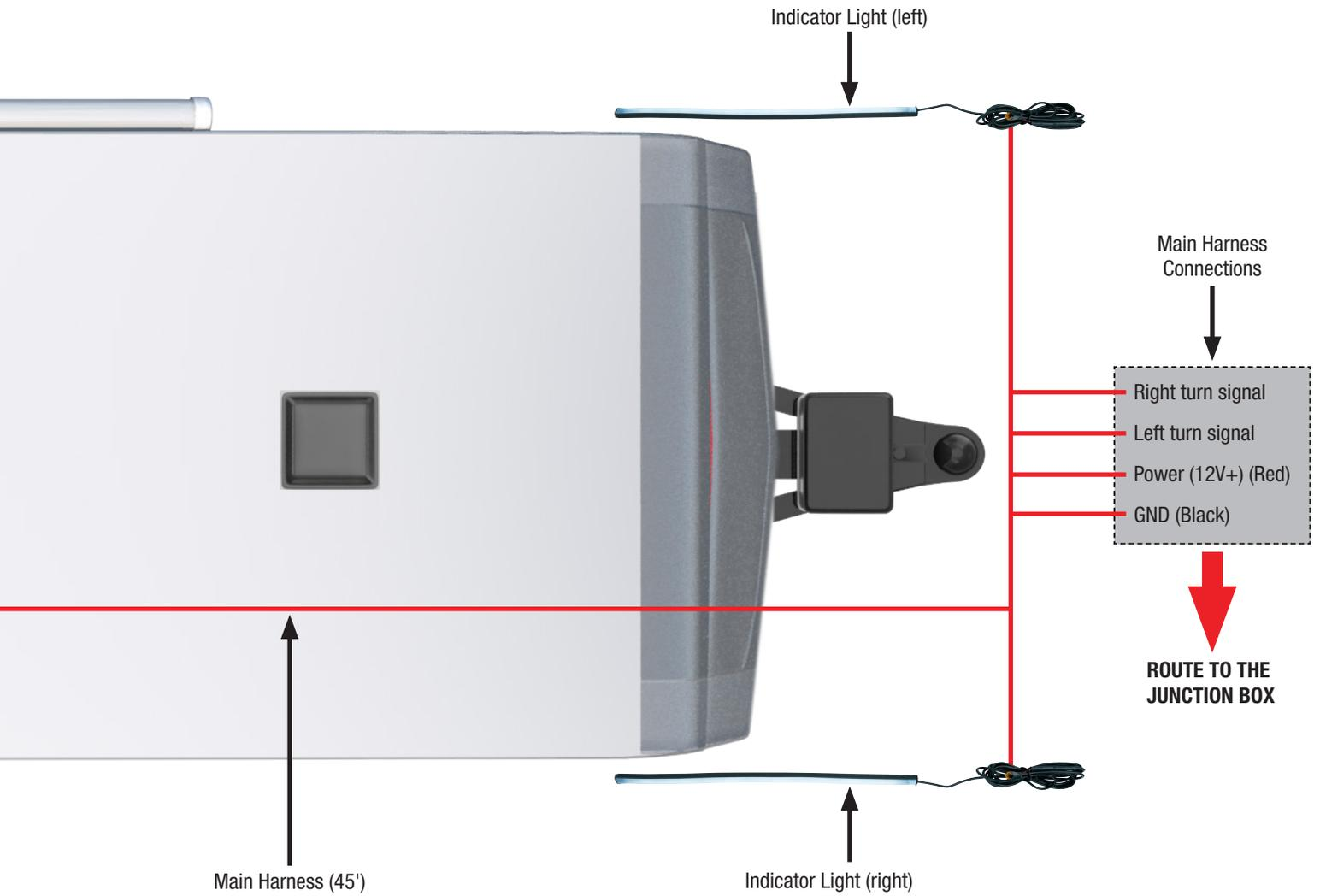
**NOTE** Use a multi-meter for identifying wires in the junction box if they are not labeled.
