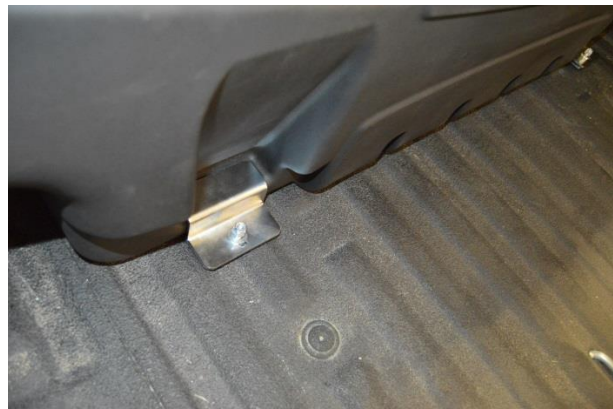
(Fig. 11) Toe clamps installed on Mounting Brackets
