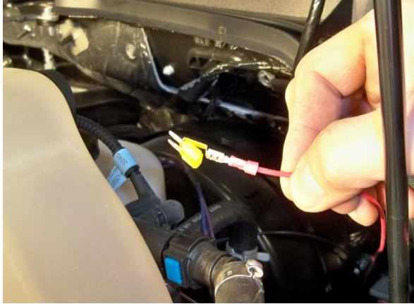
(Fig. 16) Using the supplied fuse tap, connect power Input wire to output side of 10-15 Amp fuse (Max 15 Amp).
