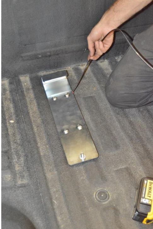
(Fig. 8) Driver's side Mounting Bracket installed. Note the ground wire attached to front inside bolt. The other end attaches to the Electronic Level Sensor.
