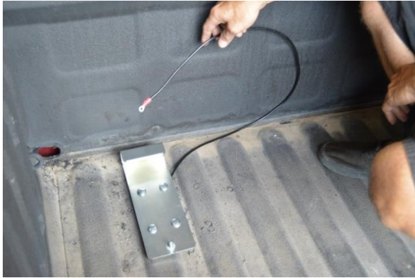
(Fig. 8) Driver's side Mounting Bracket installed. Note the ground wire attached to front inside bolt. The other end attaches to the Electronic Level Sensor on the tank.
