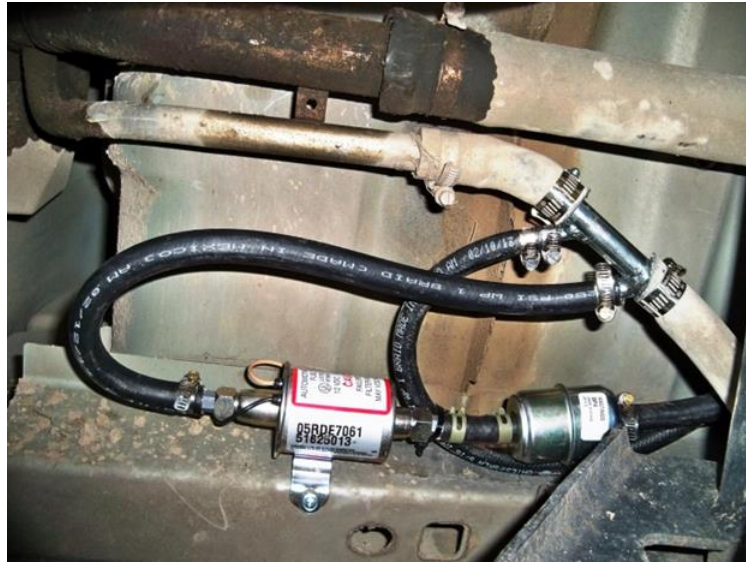
(Fig. 14) Under the vehicle, showing the Vent Line Filler Adapter installed in the vehicle's vent line.
