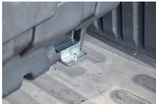
(Fig. 11) Toe clamps installed on Mounting Brackets
