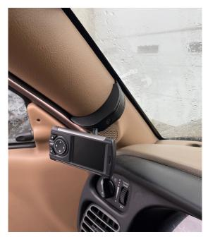
NOTE: If any of your clips holding the A-pillar trim in place are missing or broken, they may need to be replaced or the A-pillar trim may need to be secured with a screw. The added weight of the mount and display may cause the trim to fall off if the trim isn't secured.
