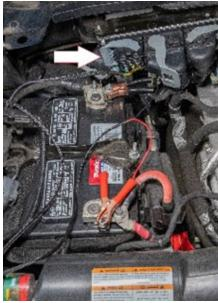
STEP 5 - Take the PCM Unlock Cable and connect it to the PCM. Make sure it is seated fully and the grey locking clamp makes an audible clicking noise (this will verify the connector is seated all the way). Next, connect the Unlock Module to the Unlock Cable (H). After, connect the tuner to the Unlock Module's OBDII port (I).
