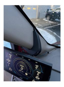
NOTE: If any of your clips holding the A-pillar trim in place are missing or broken, they may need to be replaced or the A-pillar trim may need to be secured with a screw. The added weight of the mount and display may cause the trim to fall off if the trim isn't secured.
