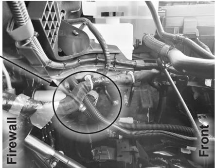
**STEP 2** - Using the image below as reference, release the red locking tab by sliding it to the left. While pressing the tab located on the top right corner of the connector hood, slide the connector hood towards the red tab (to the left) to disconnect it.
