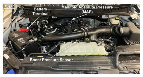
**NOTE:** For F-150's you will need to remove the engine cover. Use a 10mm socket and ratcheting wrench to remove the 2 bolts holding down the engine cover. Then pull the engine cover up and toward the front of the vehicle and set aside.
