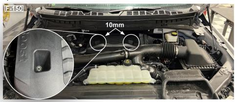
**STEP 2** - Locate the Boost Pressure Sensor connector on the charge pipe before the throttle body. Disconnect the Boost Pressure Sensor by sliding the locking tab then squeezing it. Connect both connectors to the EZX harness and lock the locking tabs.
