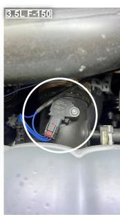
**STEP 3** - Locate the MAP sensor found on the intake manifold behind the throttle body. Disconnect the MAP sensor by sliding the locking tab then squeezing it. Connect both connectors to the EZX harness and the locking tabs.
