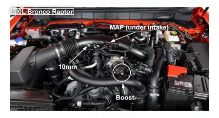
**NOTE:** The MAP connector looks just like the boost connector, but has 4 wires instead of 3.
