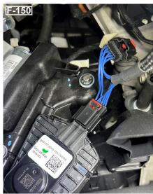
**STEP 7** - Connect the OBDII plug into the OBDII port located on the lower left side of the kick panel. Then, connect the harness to the EZX (it should click into place if completely plugged in).
