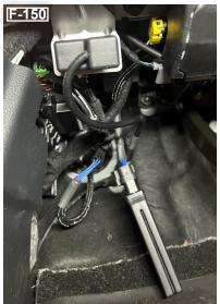
**STEP 8** - Tuck the module behind the driver's side kick panel so it is snugly held in place, then use provided zip ties to secure excess cables away from the brake and accelerator pedals, hot surfaces, and any moving components in the cab and the engine bay.
