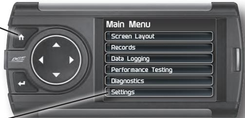
**STEP 2** - Use the Up/Down arrow buttons to scroll down to the Settings option.
